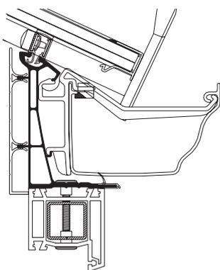
**If no reinforcing - screw up (avoiding penetration of the gutter)**
