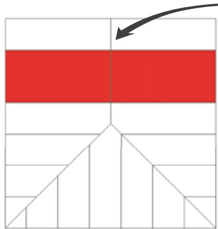
If your preferred design features a glazed panel greater than 600mm and up to the maximum of 1000mm, it is necessary to have a glazed panel each side of ridge (bars line up).
