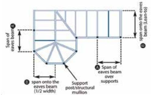
**WHERE FRAME DESIGN DOES NOT ALLOW RETRO FITMENT OF MULLIONS, ONE OPTION MAYBE TO UPGRADE FROM STANDARD EAVES BEAM TO SUPER DUTY EAVES BEAM - See p23 Appendix 4**
