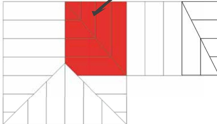
This area on a roof with a valley must be either fully glazed or fully solid
